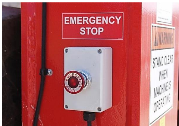
Emergency stop function on equipment and electrical control panels
