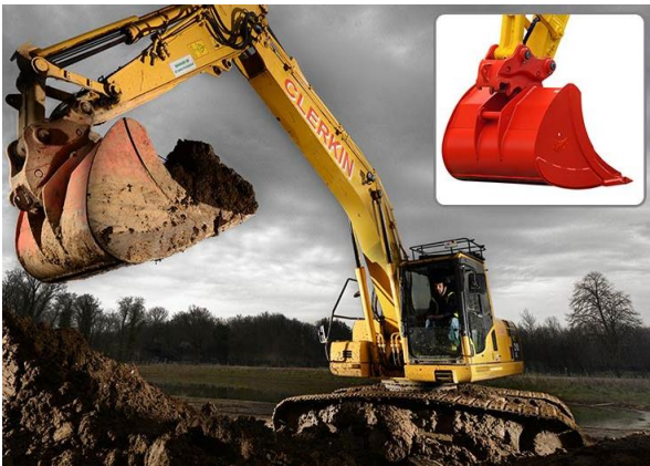
Excavator with quick hitch coupler
