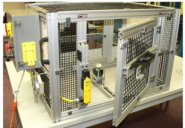
Interlocked point-of-operation guarding
