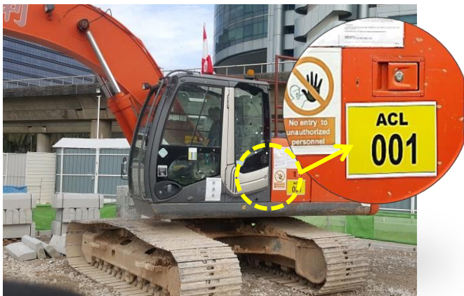
Excavator with unique identification number allocated and displayed
