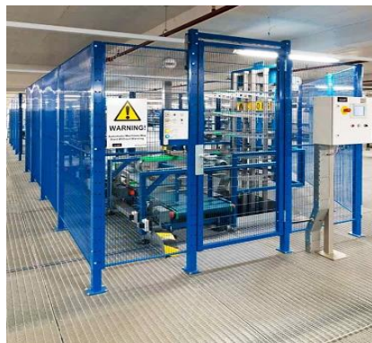
Suitable types of metal fencing and panel systems around energised equipment
