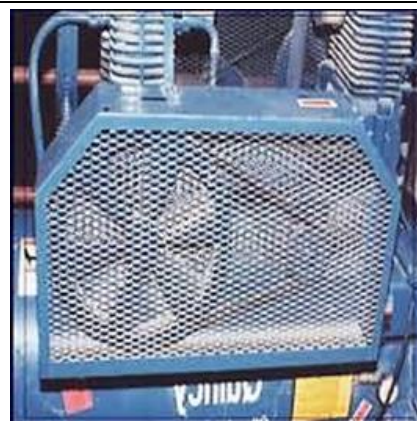
Machinery moving parts guarded with robust secure covers
