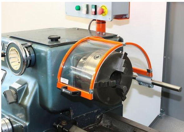
Chuck guards (interlocked) with tripping mechanism that disengages moving parts of the machine when opened or removed
