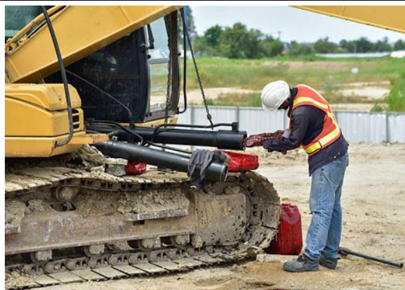
LOTO implemented for construction machinery
