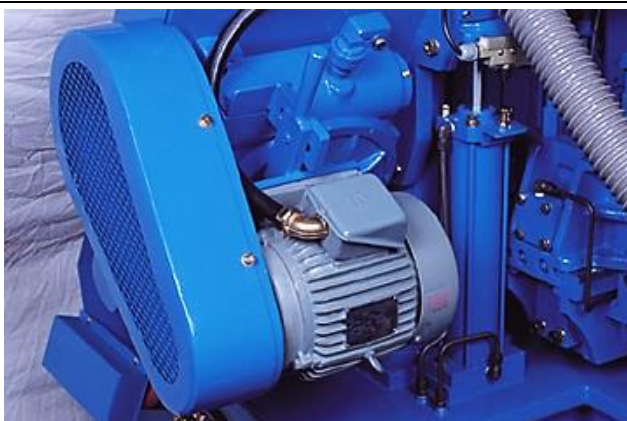
Machinery moving parts guarded with robust secure covers
