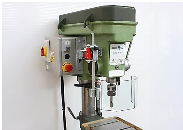
Bench drill machine with electrically interlocked guard and emergency stop function
