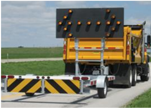
Example of truck mounted attenuator for external works
