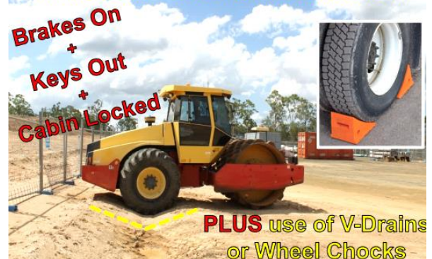
Example of stabilising vehicles with wheel chocks
