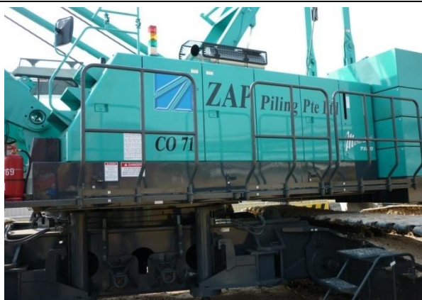
Plant fitted with guardrails to provide fall protection for personnel accessing the plant during maintenance
