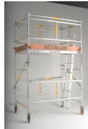
Example of a proprietary mobile scaffold tower with guardrails, toe boards, internal ladder installed at an angle and locked castors.
